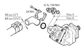
The pump can be installed in 4 positions with the angle upwards, downwards or to the side. When the angle is to the side it is an advantage if the pump can be twisted so that the suction connection is highest.
